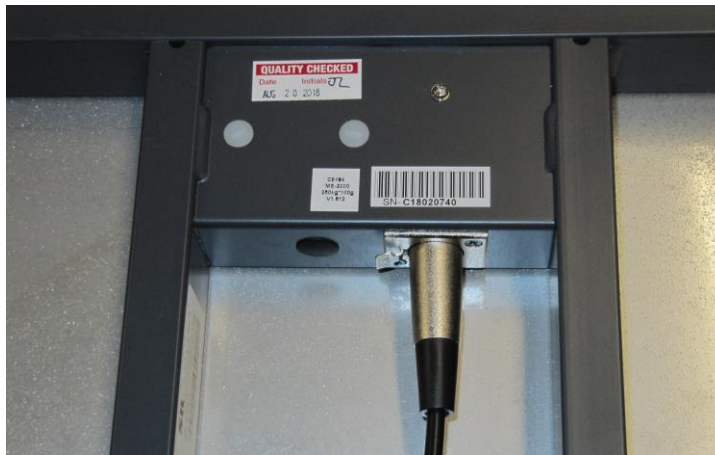
Figure 2: Cable Connection to Platform
