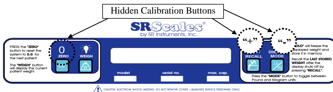
Figure 12: Calibration Hidden Buttons
