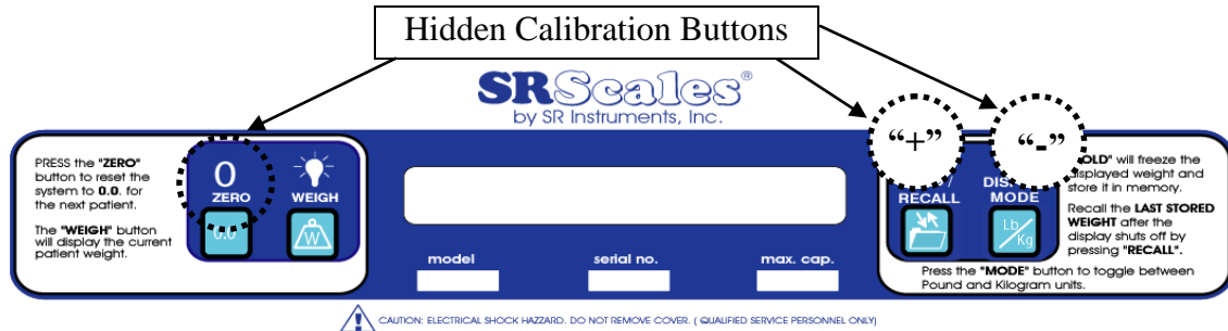
Figure 10: Calibration Hidden Buttons
