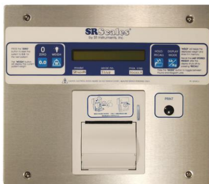
Figure 8: Front Panel Assembly
